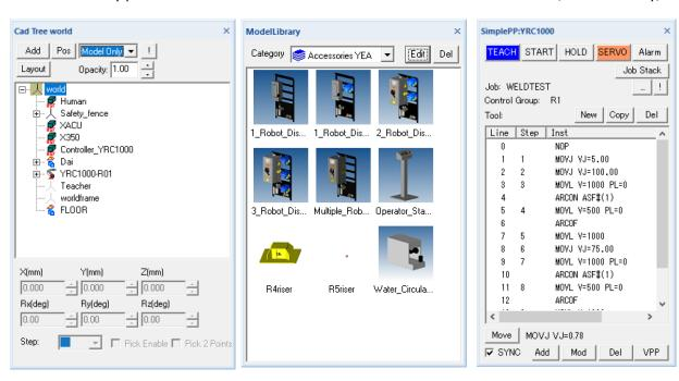
If any panel window is not appearing onscreen any longer, the best method to remedy the issue is to delete the \*.xml file in the simulation folder
